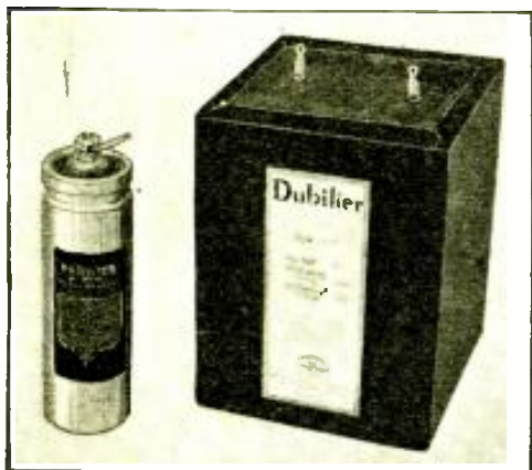
Photograph comparing the sizes of electrolytic and paper condensers, each having the same capacity—about 8 mf.
