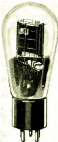
Fig. F The TS-257; a pentode.
